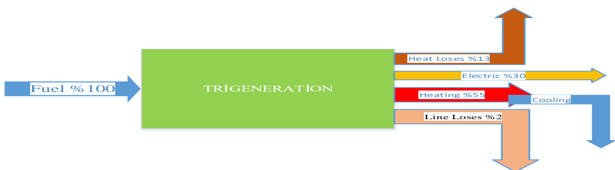
Figure 2. Schematic diagram of trigeneration system
